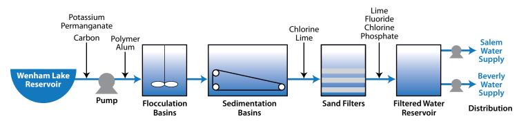
Water from the Ipswich River and the three reservoirs goes to a water filtration plant, operated 24 hours a day, 7 days a week by the Salem and Beverly Water Supply Board. The plant removes naturally occurring impurities, as required by federal regulations and good public health practices, and delivers the water to pumping stations owned by the cities of Salem and Beverly. These pumping stations deliver water
