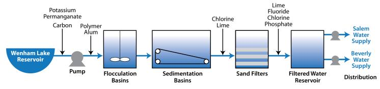
Water from the Ipswich River and the three reservoirs goes to a water filtration plant, operated 24 hours a day, 7 days a week by the Board. The plant removes naturally occurring impurities, as required by federal regulations and good public health practices, and delivers the water to pumping stations owned by the cities of Salem and Beverly. These pumping stations deliver water to your home in pipes owned
