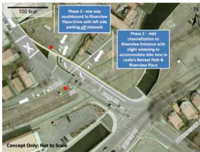
Concept for Riverview Access with Flint Street assumed one-way between Mason and Riverview Flint Street access driveway. Note bike access to Leslie's Retreat Park as an alternative to use of narrow Bridge Street segment prior to its programmed widening.
