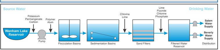
Water from the Ipswich River and the 3 reservoirs is processed by a water filtration plant, operated 24 hours a day, 7 days a week by the Board. The plant removes naturally occurring impurities from the source water, as required by federal regulations and good public health practices, and delivers the water to pumping stations owned by the cities of Salem and Beverly. These pumping stations deliver drinking water to your home in pipes owned and maintained by each city water department.
