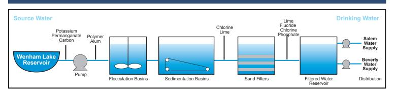
Water from the Ipswich River and the 3 reservoirs is processed by a water filtration plant, operated 24 hours per day, 7 days per week by the Board. The plant removes naturally occurring impurities from the source water, as required by federal regulations and good public health practices, and delivers the water to pumping stations owned by the cities
