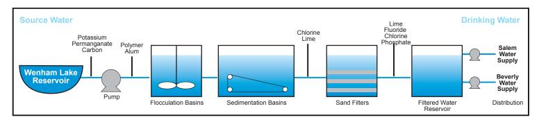
Water from the Ipswich River and the 3 reservoirs is processed by a water filtration plant, operated 24 hours per day, 7 days per week by the Board. The plant removes naturally occurring impurities from the source water, as required by federal regulations and good public health practices, and delivers the water to pumping stations owned by the cities of Salem and Beverly. These pumping stations deliver drinking water to your home in pipes owned and maintained by each city water department.
