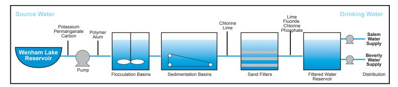
Water from the Ipswich River and the 3 reservoirs is processed by a water filtration plant, operated 24 hours per day, 7 days per week by the Board. The plant removes naturally occurring impurities from the source water, as required by federal regulations and good public health practices, and delivers the water to pumping stations owned by the cities
