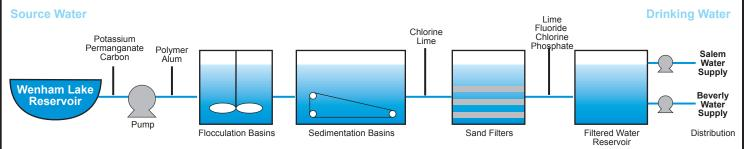
Water from the Ipswich River and the 3 reservoirs is processed by a water filtration plant, operated 24 hours per day, 7 days per week by the Board. The plant removes naturally occurring impurities from the source water, as required by federal regulations and good public health practices, and delivers the water to pumping stations owned by the cities of Salem and Beverly. These pumping stations deliver drinking water to your home in pipes owned and maintained by each city water department.
