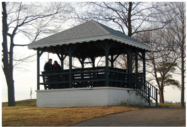
6. Pavilion "B" (bandstand) with built in benches, modified 'pennant' trim, concrete floor and foundation, concrete steps and iron handrails. 2018
